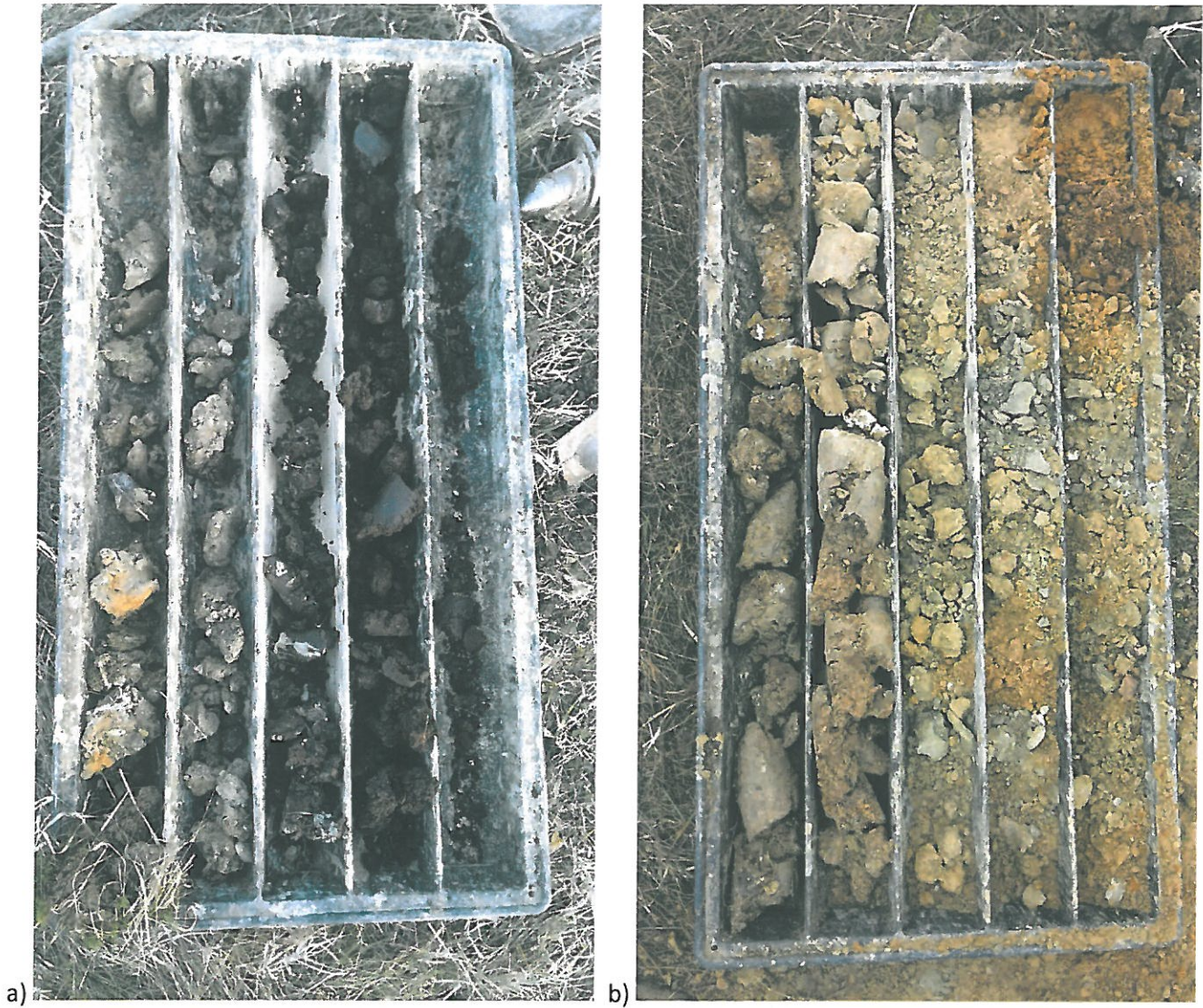
Fig. 20 - Coloana litologica foraj M2, adancimea 0 m - 5 m (a) si 6 m -10 m (b)
