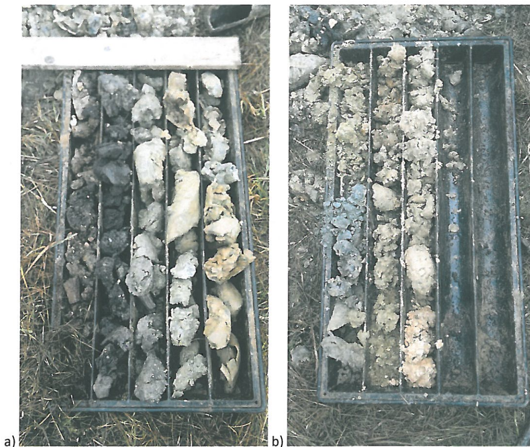
Fig. 25 - Coloana litologica foraj M3, adancimea 0 m - 5 m (a) si 6 m - 8 m (b)
